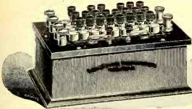
Commercial Form of Wheatstone Bridge for Measuring Resistance Similar to the Type Here Described.
